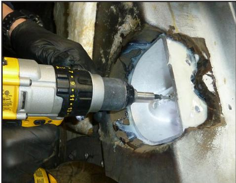
Install the plug & use a #10 wood screw to secure the plug in position. Wipe up excess adhesive with a gloved finger or spreader.
