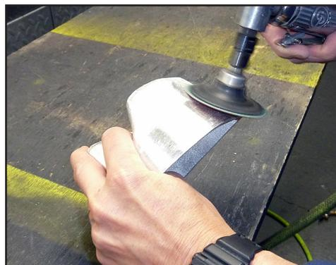
Thoroughly grind the outside surface of the plug with a 50 grit Roloc® disk to make the aluminum receptive to PlastiFix® adhesive.
