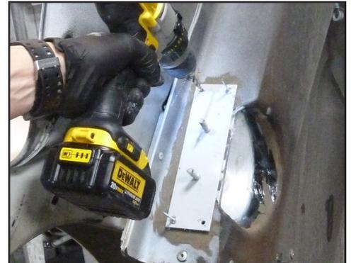
With a rivet temporarily placed in the first hole as a guide, drill the remaining rivet holes. Remove the plate, bolts, and rivet.
