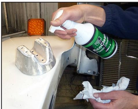
Clean the outside of the reinforcing plugs with 1001-4 Eco-Prep Plastic Cleaner.
