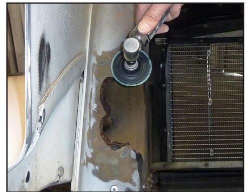
Grind the flat area where the plates will be bonded with a 50 grit Roloc® disk, then blow dust free.
