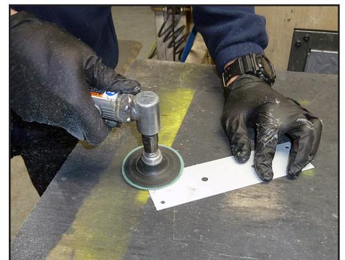
Grind the paint off of one side of the bearing plate to improve adhesion. Blow dust free. Do not clean with 1001-4 Eco-Clean.
