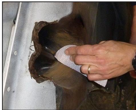
HAND SAND the inside of the pockets with 60 to 80 grit sand paper to roughen the surface and remove ALL paint.
