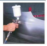
Step 2. Agitate Bumper & Cladding Coat Adhesion Primer and strain into a paint gun. No reducer or activator is required. Apply with a 0.8-1.3mm basecoat gun for fine atomization. Both ambient and surface temperatures should be between 65°F (18°C) and 95°F (35°C). Apply one or two light to medium coats using 25-35 psi at the gun to achieve hide. Do not try to flow Bumper & Cladding Coat out; it will appear slightly rough until dry. Allow five minutes of flash time between coats.
