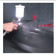
Step 1. Clean plastic with 1000 Super Prep or 1001 EcoPrep Plastic Cleaner. Spray on a heavy, wet coat in an area about one foot square, wait a few seconds, then wipe in one direction with a clean cloth. On raw TPO plastic surfaces, no sanding or scuffing of surface required.
