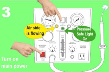
Open nitrogen tank valve & set regulator to 15 psi
