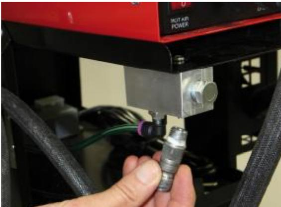
2. Install your shop's quick disconnect plug into the bottom inlet port of the cart's air manifold.
