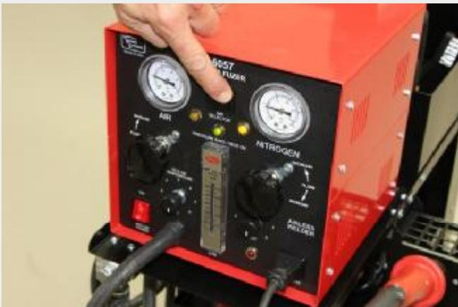
3. Switch the air selector to the nitrogen side briefly to purge the nitrogen from the lines. Immediately switch back to air to continue cooling the heating element.
