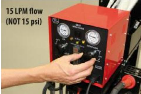
9. Adjust fine flow control on the nitrogen (right) side so the flow meter reads 15 LPM. You should feel nitrogen gas coming from the torch.
