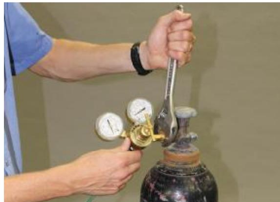
5. Screw the nitrogen regulator into the tank. Do NOT use teflon tape. Tighten securely.
