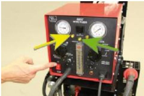
5. Plug in and turn on power strip. Turn hot air power switch on. Verify that the yellow light on the "air" side and the green "pressure safe" lights are glowing.
