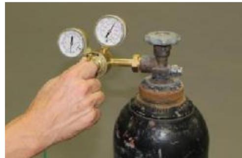
8. Turn pressure screw clockwise until the outlet side gauge shows 15 psi.
