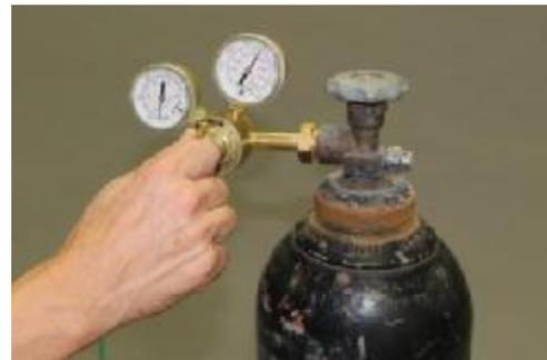
8. Turn pressure screw clockwise until the outlet side gauge shows 15 psi.
