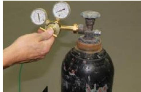
6. To turn on the nitrogen, back out the pressure screw on the nitrogen tank regulator to prevent possible overpressure from damaging downstream components or the tank regulator.
