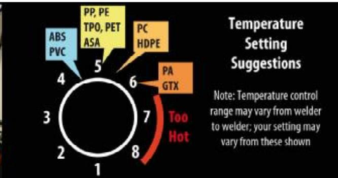
11. Turn the temperature control dial to the proper level for the plastic you are working with. Let the welder warm up for five minutes before use.
