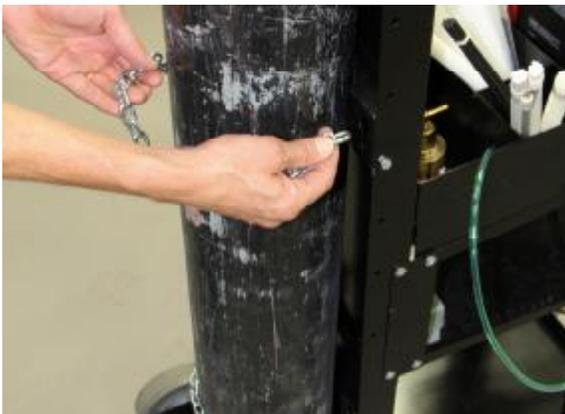
4. Install nitrogen tank (argon or argon/CO2 may also be used). Install included safety chains around tank. Adjust height of top tank cradle if necessary.
