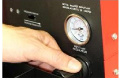
2. Set inlet pressure regulator on back of the welder to 15 psi.
