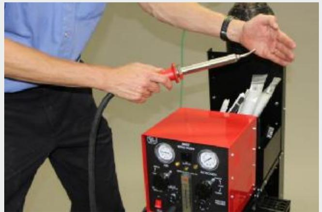
4. Let the air flow for at least 10 minutes or until the air coming from the nozzle is completely cool to the touch. Shut off the hot air power switch, turn off the power strip, and unhook the shop air line.
