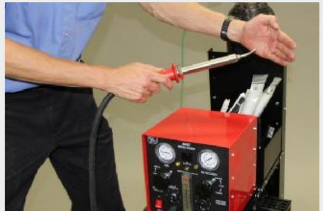
4. Let the air flow for at least 10 minutes or until the air coming from the nozzle is completely cool to the touch. Shut off the hot air power switch, turn off the power strip, and unhook the shop air line.
