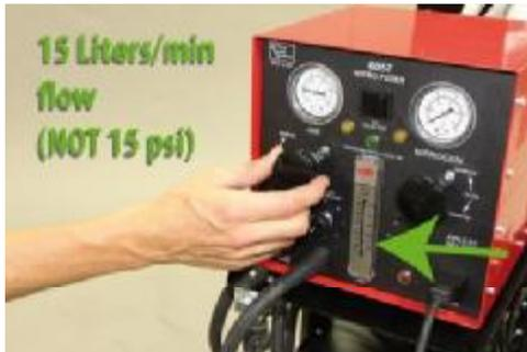
3. Adjust fine flow control on the air (left) side so the flow meter reads 15 LPM. You should feel air coming from the torch.
