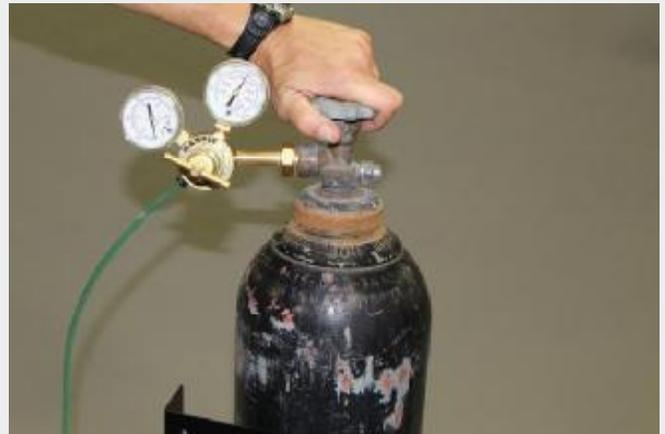
2. Close the nitrogen tank valve. This will prevent any downstream leaks from draining the tank while the welder is off.
