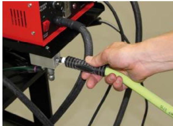
3. A short whip hose may be attached at the front of the air manifold if desired to power your die grinder and sander.
