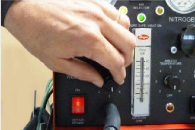
1. Turn the hot air temperature control to Level 1. This will shut down current flow to the heating element. Allow the air to flow and cool the element.
