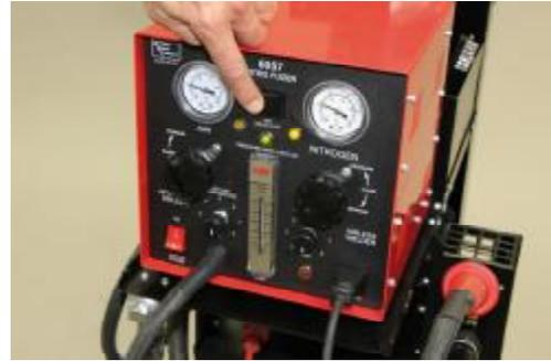
10. Switch the air selector back and forth between air and nitrogen, making sure that the yellow lights indicate which side is flowing, that the green pressure safe light is glowing on both sides, and that you have flow from the torch on both sides. Leave on air at all times except when you're actually welding.
