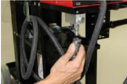
1. Connect clean, dry, oil-free shop air to air inlet. Supply pressure should be set between 60-120 psi.
