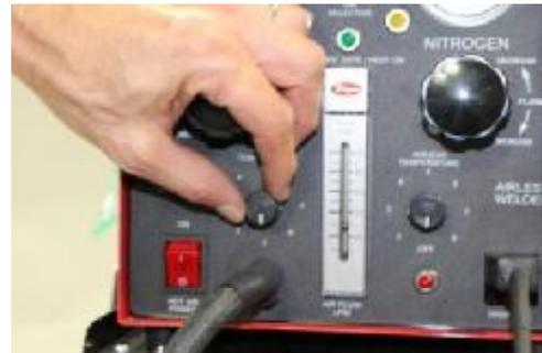
4. Adjust hot air temperature control to Level 1 to prevent any current flow to heating element.
