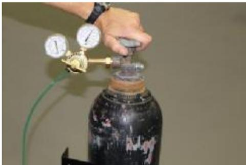
7. Open nitrogen tank valve slowly. Check that the tank gauge needle shows some pressure in the tank.
