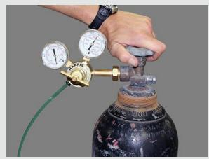
2. Close the nitrogen tank valve. This will prevent any downstream bleed-off from draining the tank while the welder is off.
