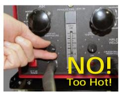
12. Do NOT leave on heat level 7 or 8 for any length of time because you will overheat the element! These settings are appropriate for higher airflow settings and thicker plastics., NOT for thin plastics like used for most automotive parts.
