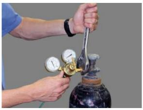
Screw the nitrogen regulator into the tank. Do NOT use teflon tape. Tighten securely.
