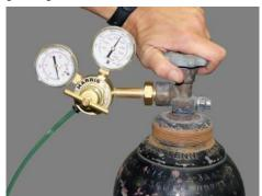
7. Crack open nitrogen tank valve slowly. Confirm that the tank gauge needle shows pressure in the tank.
