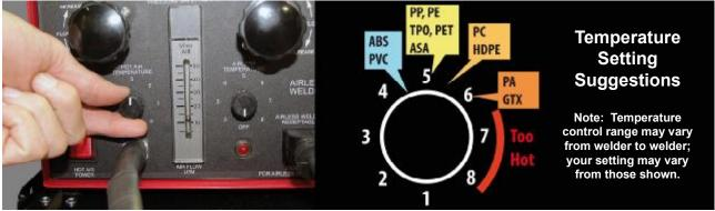
11. Turn the temperature control dial to the proper level for the plastic you are working with. Let the welder warm up for five minutes before use.
