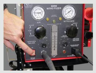
4. Shut off main power and stop airflow by unscrewing the air regulator knob until loose. Disconnect air supply and unplug from the wall.
