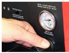
2. Set inlet pressure regulator on back of the welder to 15-20 psi.
