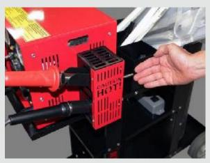
3. Let the air flow for 10 minutes or until the air flowing from the welding tip is completely cold.
