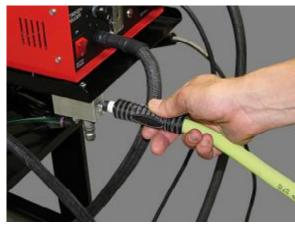
3. A short whip hose may be attached at the front of the air manifold if desired to power your die grinder and sander.
