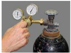
Turn pressure screw clockwise until the outlet side gauge shows 15 psi.
