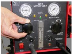
3. Adjust fine flow control on the air (left) side so the flow meter reads 12 LPM. You should feel air coming from the torch.
