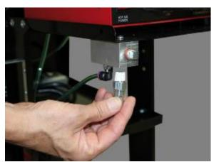
Install your shop's quick disconnect plug into the bottom inlet port of the cart's air manifold.
