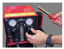
Remove torch from the holster to switch to nitrogen. Adjust the pressure on the nitrogen (right) side so the flow meter reads 12 LPM. You should feel nitrogen gas coming from the torch.
