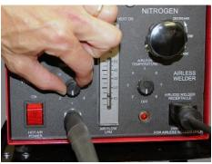
4. Adjust hot air temperature control to Level 1 to prevent any current flow to heating element.
