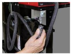
1. Connect clean, dry, oil-free shop air to air inlet. Supply pressure should be set between 60-120 psi.
