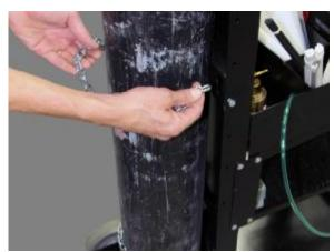
Install nitrogen tank (argon or argon/CO2 may also be used). Install included safety chains around tank. Adjust height of top tank cradle if necessary.
