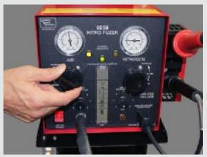
1. Place torch in the upper holster and turn the air temperature control to Level 1 to shut down the power to the heating element. Turn up the airflow to >25 LPM to speed the cooling process.
