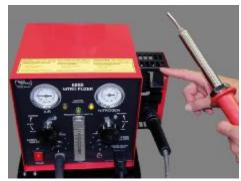
10. Switch the air selector back and forth between air and nitrogen, making sure that the yellow lights indicate which side is flowing, that the green pressure safe light is glowing on both sides, and that you have flow from the torch on both sides. Leave on air at all times except when you're actually welding.
