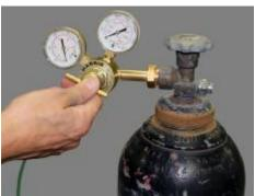
6. To turn on the nitrogen, back out the pressure screw on the nitrogen tank regulator to prevent overpressure from damaging the tank regulator or downstream components.
