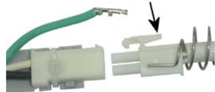
Push the locking lever to unhook the ceramic heater core and unplug the ceramic heater core from the power lines.
