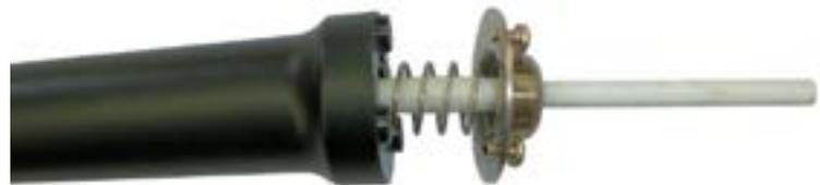
Remove the 3 screws that hold the base plate to the handle and slide the handle away from the ceramic core assembly.
