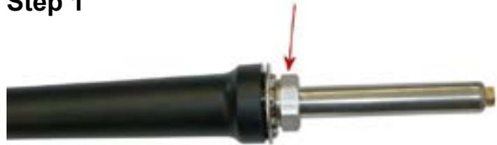
Remove the large nut at the base of the barrel and slide the barrel off of the assembly.
