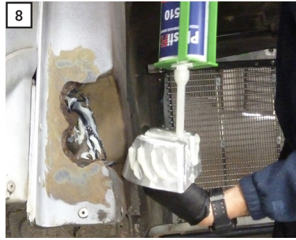
8 Generously coat the plug and socket with enough PlastiFix adhesive to fill any gaps between the plug and the pocket.
