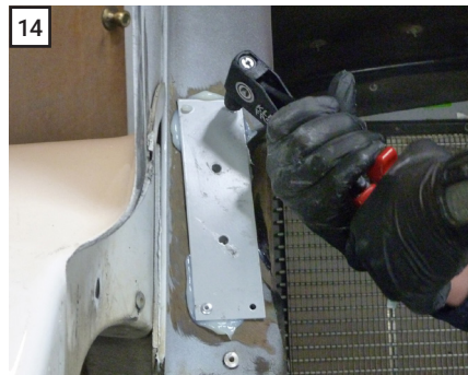
14 While pushing firmly down on the bearing plate, rivet the plate into place using four 3/16" rivets, one in each corner.
