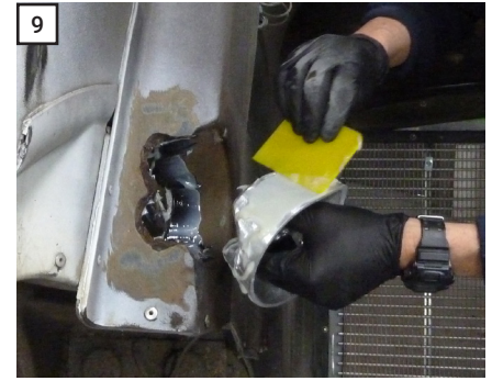
9 Spread the adhesive evenly over the plug and inside the socket. Working time is about 15 minutes at room temperature.
