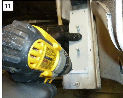
11 Using two 5/16" x 2" bolts as a guide for the bearing plate, drill the first 3/16" rivet hole into the hood. Note: The plates are identical.
