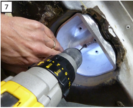
7 Drill a 1/8" pilot hole into the plastic using the middle plug hole as a guide. Use the correct DRVR or PASS plug, they are different!
