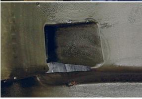
3. Test fit the casting to the pocket and trace around the perimeter with a permanent marker. Cut away as much of the flange as needed to make the reinforcement fit all the way down into the pocket.
