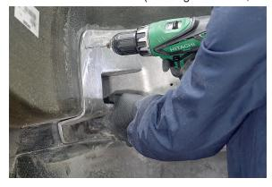
10. Drill all seven (7) hole locations and remove the dust using compressed air or a cloth dampened with EcoPrep<sup>™</sup> or Super Prep<sup>™</sup> plastic cleaner. Make sure the area is <u>completely</u> dry before proceeding.
