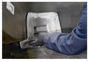
9. Using a permanent marker or a drill, mark the hole locations for the screws. (Marking with a drill, shown.)
