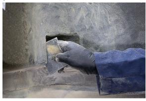
Clean the outside of the aluminum castings with 1001-4 Eco-Prep<sup>™</sup> plastic cleaner or 1000-A Super Prep<sup>™</sup> plastic cleaner.
