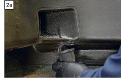
Using the trim saw, cut away the edge of the hood spring pocket to allow the casting center to clear the hood. Leave as much material as possible to keep the maximum bond area between the hood and the casting.
