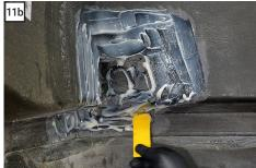
Immediately apply a generous layer of 2510 PlastiFix over the mating surface of the casting. Apply the adhesive in rows to allow air to escape when pressing the parts together. There should be enough adhesive applied to the casting to cause some of it to squeeze out when the casting is screwed into place.
