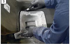
Test fit the casting to the pocket and trace around the perimeter with a permanent marker. Cut away as much of the flange as needed to make the reinforcement fit all the way down into the pocket.
