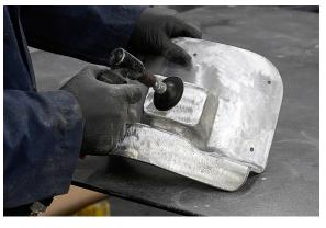
8. Test fit the casting and push it firmly into place. It should be in contact with the hood everywhere, however short gaps up to approximately 1/8" are acceptable but will need to be completely filled with PlastiFix<sup>®</sup> adhesive. If it doesn't sit all the way down into the pocket, sand or grind the interfering areas of the hood or casting and test fit again. Repeat this until you're confident the casting is bottomed out in the pocket.
