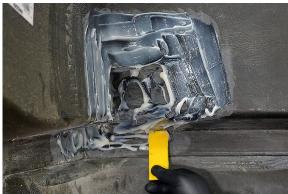
12. Immediately apply a generous layer of 2510 PlastiFix® over the mating surface of the casting. Apply the adhesive in rows to allow air to escape when pressing the parts together. There should be enough adhesive applied to the casting to cause some of it to squeeze out when the casting is screwed into place.
