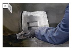
Test fit the casting and push it firmly into place. It should be in contact with the hood everywhere, however short gaps up to approximately 1/8" are acceptable but will need to be completely filled with PlastiFix adhesive. If it doesn't sit all the way down into the pocket, sand or grind the interfering areas of the hood or casting and test fit again. Repeat this until you're confident the casting is bottomed out in the pocket.
