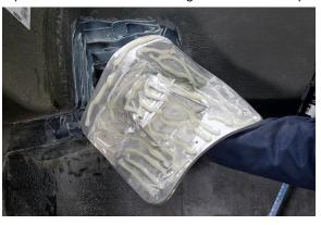
13. Install the casting and secure it into position loosely with the included screws. DO NOT TIGHTEN the screws until all screws are in place and the casting is seated into the pocket correctly. <u>Hand tighten</u> the screws only until firmly snug. If the screws are installed too tightly, too much adhesive will squeeze out, starving the joint and weakening the bond.
