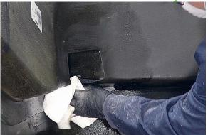
2. Using the trim saw, cut away the edge of the hood spring pocket to allow the casting center to clear the hood. Leave as much material as possible to keep the maximum bond area between the hood and the casting.
