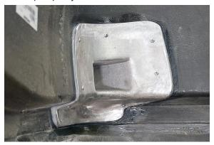
16. When fully cured, install the OEM eyebolts into the casting with low or medium strength threadlocker to prevent galvanic corrosion between the eyebolt and the casting. Use a nut and lockwasher on the inside of the pocket to lock the eyebolt into position.
