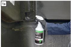
Using 1001-4 EcoPrep plastic cleaner, clean the spring hood pocket and the surrounding area where the reinforcing plate will be attached.
