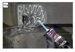
Apply a generous layer of 2510 PlastiFix evenly over the mating surface of the hood. Spread the adhesive with a body spreader and work it into the sanding scratches. Work quickly because the adhesive working time is 15 minutes at 68°F (20°C).
