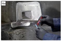
When fully cured, install the OEM eyebolts into the casting with low or medium strength threadlocker to prevent galvanic corrosion between the eyebolt and the casting. Use a nut and lockwasher on the inside of the pocket to lock the eyebolt into position.
