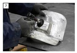
Thoroughly grind the bonding surface with a 50 grit Roloc™ disc to make it receptive to 2510 PlastiFix adhesive.
