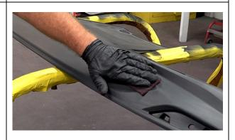
8. Fill an HVLP gravity-feed spray gun with Flextex VT reduced to match the texture determined in Step 2. Gun nozzle size, needle setting, and air pressure are all variables to be adjusted to fine-tune grain size. Adjust gun settings on a sprayout card before applying texture to the part.
