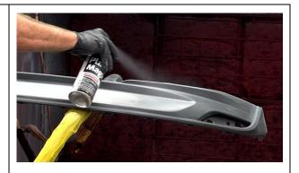
Spray 3043 All Seasons Black Jack waterborne primer surfacer (or your desired primer surfacer). Apply two medium wet coats, blending out from the repair area into the original texture and allowing some flash time between coats.
