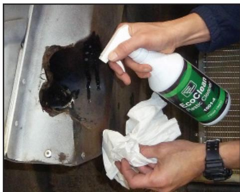
Clean both pockets and the surrounding area where the plate will be bonded in the hood with 1001-4 Eco-Clean Plastic Cleaner.
