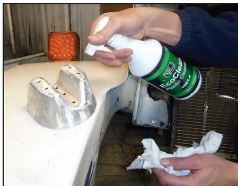
Clean the outside of the reinforcing plugs with 1001-4 Eco-Clean Plastic Cleaner.
