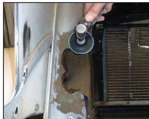
Grind the flat area where the plates will be bonded with a 50 grit Roloc® disk, then blow dust free.
