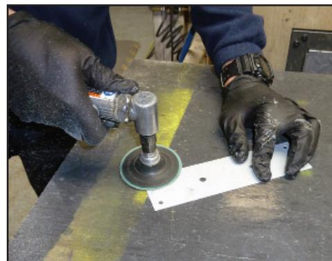
Grind the paint off of one side of the bearing plate to improve adhesion. Blow dust free. Do not clean with 1001-4 Eco-Clean.
