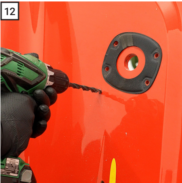
12 Counter-bore the 1/4" hole, 1/4" deep with a 3/8" drill bit to provide clearance for the bolt's shoulder.
