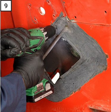
9 Drill the marked holes with a 5/32" drill bit. Drill through to the outside of the hood only in the location shown above.
