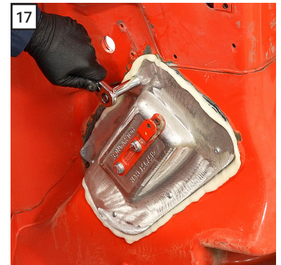
17 Install the casting onto the hood using the screws, elevator bolt, and nut. Apply just enough torque to snug the casting in place.
