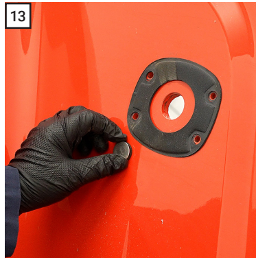
13 Tap the elevator bolt with rubber washer into the hole.
