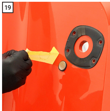
19 Remove the tape and wipe away any adhesive that may have squeezed through
