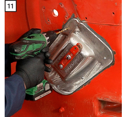
11 Loosely screw the casting to the hood. Using gentle pressure and high speed to reduce tear-out, drill a 1/4" hole through the hood at the location shown.
