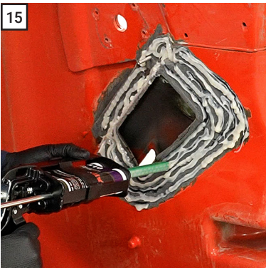
15 Remove the casting then apply half a cartridge of 2510 PlastiFix adhesive to the hood.
