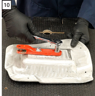
10 Apply blue thread locker to the bolts and fasten the forked bracket to the casting.
